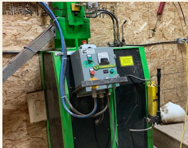
The funding from the Momentum Fund helped Ferme Amico buy a pelleting machine to turn its chicken compost into easy-to-use pellets.
